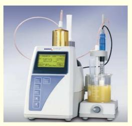
New and used insulating materials can contain basic constituents which are present as additives. The relative content of these materials can be determined by titration with acids. The bas number is the measure of the amount of basic substances in the oil always under the conditions of the test. Acid number is expressed by potassium hydroxide in mg required to neutralize free fatty acid in 1g of oil.
